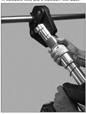
Press Ring/Vic-Press Adapter Jaw Assembly for 1½-inch/48.3-mm and 2-inch/60.3-mm Sizes
