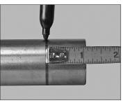
1. When using a ruler or tape measure, refer to the "Vic-Press Schedule 10S Insertion Depth Requirements" table below. Measure back from the pipe end. Place a mark around the pipe circumference with a marker or paint stick, as shown above.
