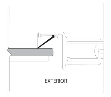
13 Carefully silicone the seam between the walls and the wall jambs as well as the curb and threshold on the inside of the shower.
