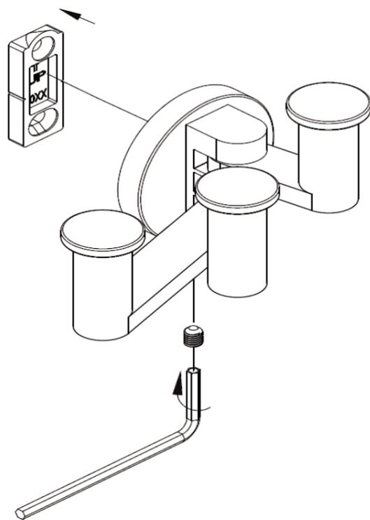
② ALIGN MOUNTING BRACKETS AND MARK LOCATION
