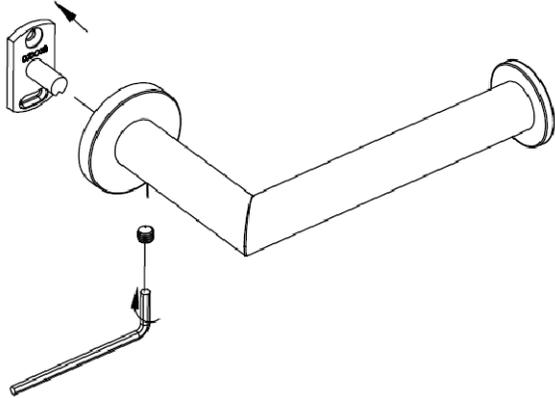
② ALIGN MOUNTING BRACKETS AND MARK LOCATION
