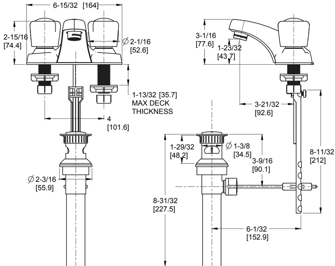
$\varnothing 1$  Min to  $\varnothing 1\frac{1}{2}$  Max. Deck Hole Openings
