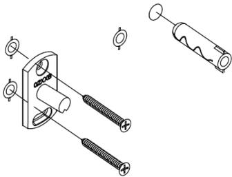
5 INSTALL PRODUCT ONTO BRACKETS REGISTER ROSETTE ONTO POST AND PRESS LIGHTLY DURING INSTALLATION.
