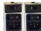
Sliding switch for 115v or 230v on dual voltage models
