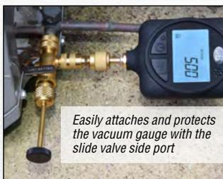
Easily attaches and protects the vacuum gauge with the slide valve side port
