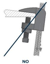
Improper installation with load at angle to threaded rod.
