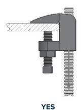
Proper installation with load in line with threaded rod.
