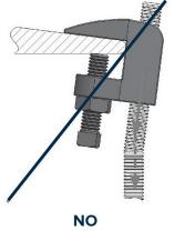
Improper installation with bent threaded rod.
