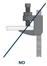
Improper installation with beam clam in reverse direction. \*3/8" only size acceptable for reverse installation (max load 200 lbs).
