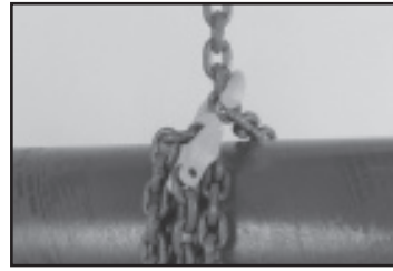
Fig. 4. "A GrabiQ C-Grab used at the bottom of the sling as an adjustable sliding choker."
