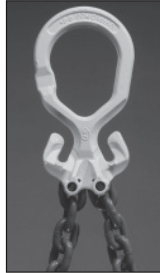
Fig. 1. The GrabiQ Master Grab combines a master link, master link connectors for two legs of chain, and two shortening hooks into a single fitting. The shortening hook can also be used to create loop legs.
