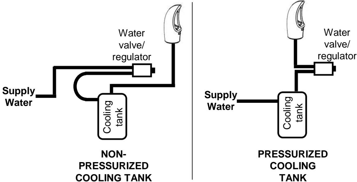
1. With the cooler top removed, find the tube going from the cooling tank outlet to the valve. The TEE fitting (supplied) will need to connect between the cooling tank and valve.
