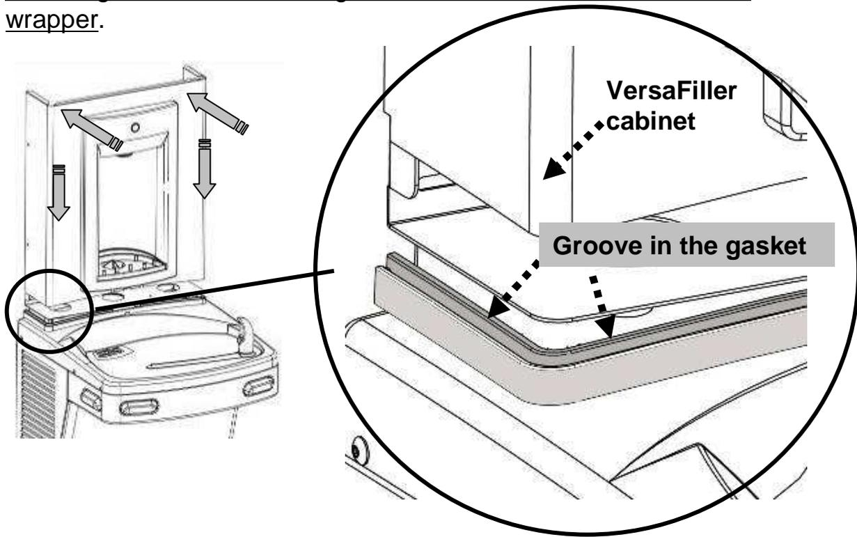
6. Attach VersaFiller assembly and top cap to the frame using the six (6) torx screws.
