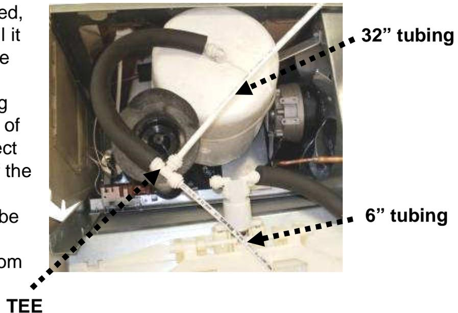
4. Route the TEE and tubing under the waste drain and connect the 6" length to the water valve elbow.
