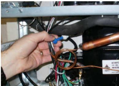
Next, insert end of tube into fitting.
