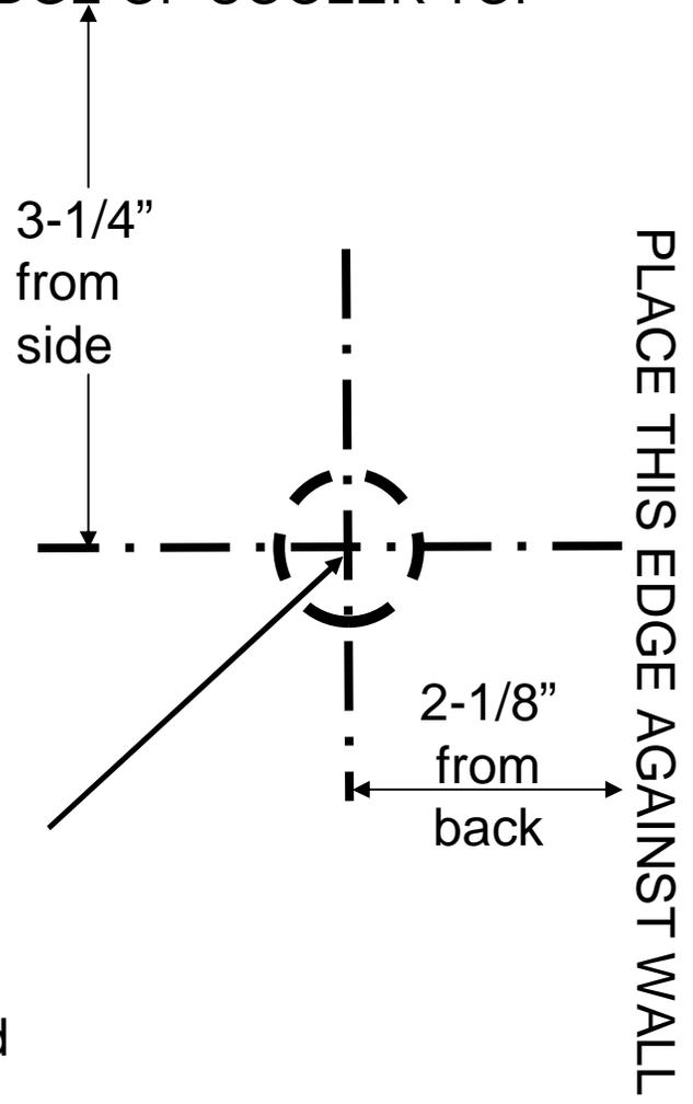
Mark this center point on the top. Remove the top from the cooler. Then drill a 3/8 hole through the top at the marked center point.
