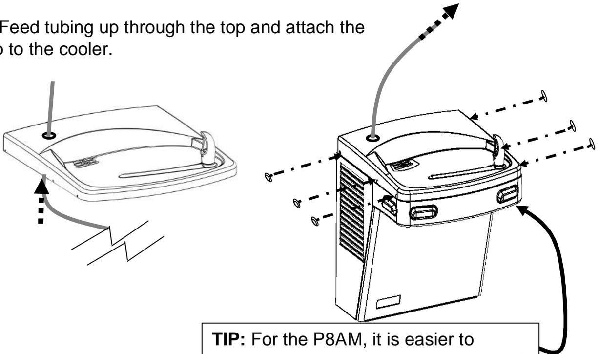
**TIP:** For the P8AM, it is easier to connect the outlet tube to the bubbler if the front nose is removed.
