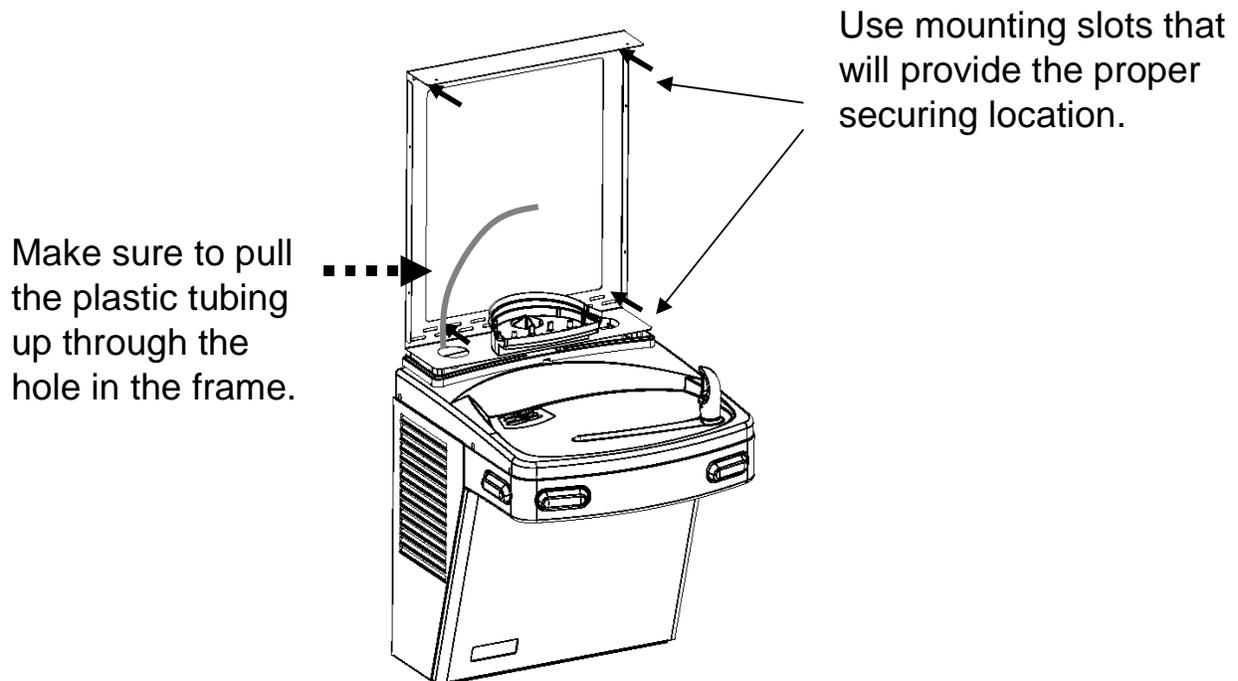
3. Secure frame to the wall with fasteners (not provided). Pull plastic tubing up through the hole in the frame.
