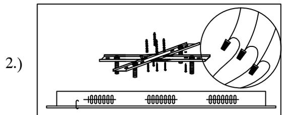
2.) Step.2: Wire fixture to wires in outlet box. Green wire is for Ground.
