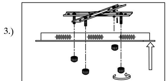
3.) Step.3: Screw finials (D) onto mounting bracket (A) until canopy is flush with ceiling.
