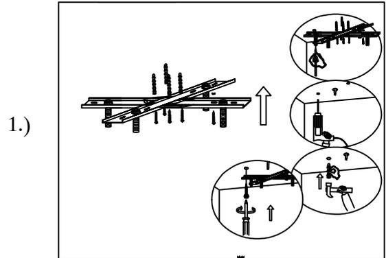
1.) Step.1: Remove mounting bracket (A) from Canopy (C) to install to electrical box
