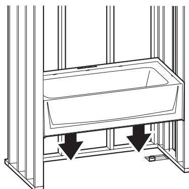
Lift and place the base into framing.
