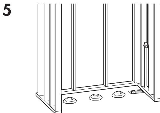
Install drain assembly per manufacturer's instructions. If desired, spread foundation material. When using foundation materials, the following applies: Mix foundation material. Place three or four mounds of plaster on the subfloor around but away from drain hole. The mounds should be placed high enough so that when the unit is set, it will cause the plaster to displace and spread.
