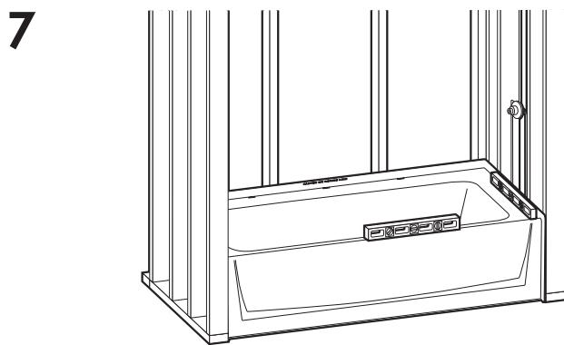
Tap down until level. Level lengthwise and widthwise using 3 ft. (915mm) level by shimming or depressing foundation materials. The unit must be set level.
