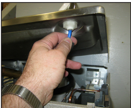
Remove Bubbler Water Line
