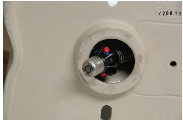
Figure 18 – Camera Head with Ball Guide in Turn
