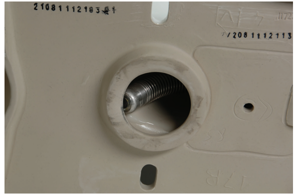
Figure 17 – Camera Head Blocked in Turn
