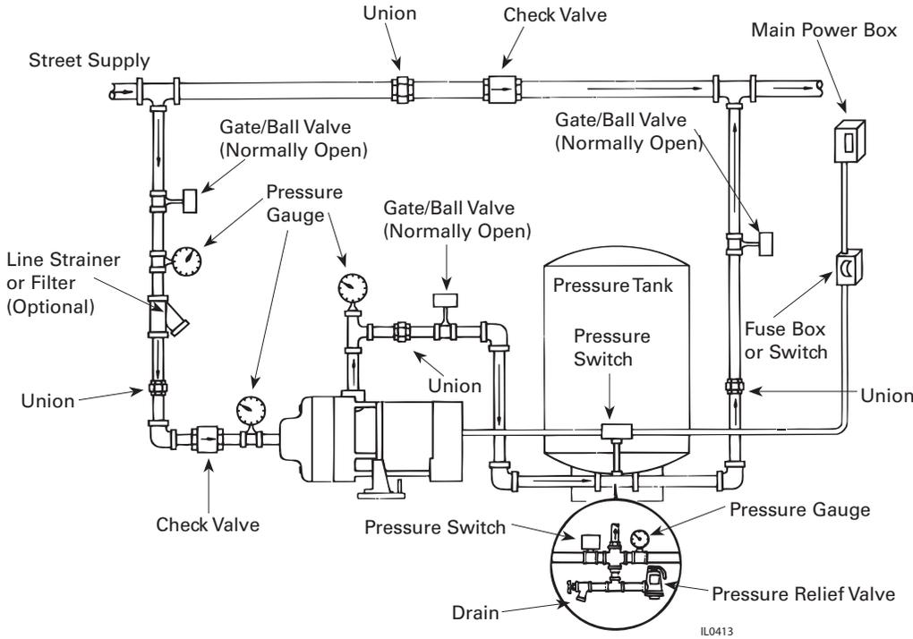
To size pressure tank properly, match the drawdown of the tank to the capacity of the pump.
