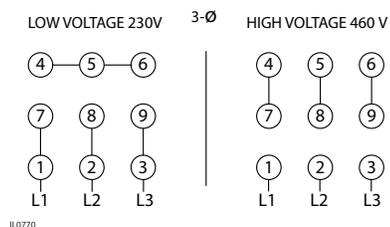
Figure 9 - Wiring Diagram for Three Phase
