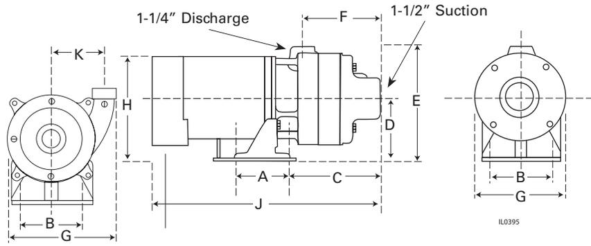
Figure 4 - CJ101B Two and Three Stage Booster Pump
