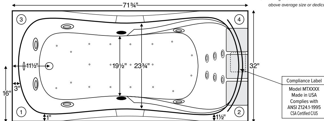
Numbered areas on tub deck represent possible locations to install cleaning systems, faucets and other fixtures.
