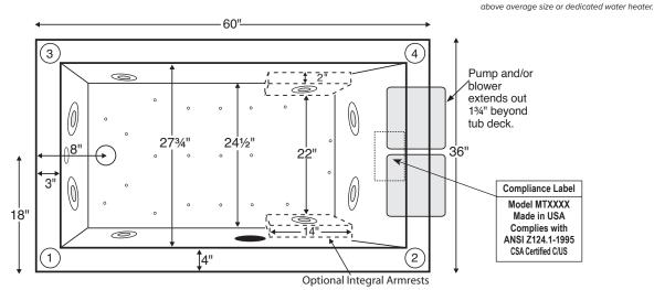
Numbered areas on tub deck represent possible locations to install cleaning systems, faucets and other fixtures. Pump extends out approximately 1 3/4" beyond tub deck.
