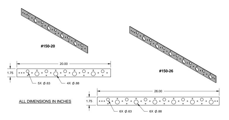
The HOLDRITE<sup>®</sup> #150-20 and #150-26 are Copper-Bonded<sup>™</sup> steel brackets for support of ½" and ¾" pipes on 4" or 8" centers. The #150-20 & #150-26 position copper water supplies for sinks, water closets, and other fixtures. When soldering, heat the pipe, not the bracket.
