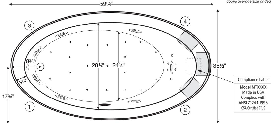
Numbered areas outside of tub represent possible stub-out locations for cleaning systems and Breda valves.
