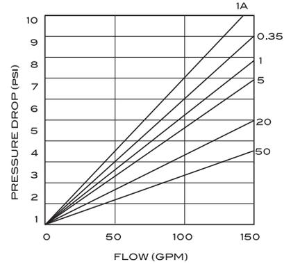
Note: Pressure drop data shown above include filter housing and cartridge.
