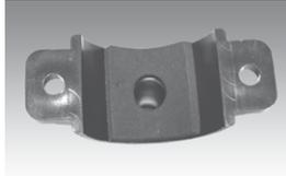
**Step C** – The drain saddle must be installed at least 1 1/2" above the nut of the P-Trap elbow or cross bar from the garbage disposal to insure proper drainage. Using the 1/4" drill bit, drill into the drain pipe at best available location as specified above, for drain saddle installation. Take extreme caution to only drill through one side of the drain pipe.
