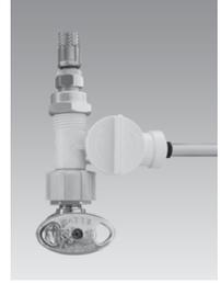
**Step B** – Connect the green tube from the RO module to the Adapt-A-Valve™ that is connected to the angle stop valve. Leave enough tube so it is not kinked and cut the tube to the desired length.
