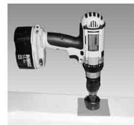
**Step C** – Using a 1¼" hole saw, proceed to drill the large hole. Keep drill speed on the slowest speed and use lubricating oil or liquid soap to keep the hole saw cool during cutting.
