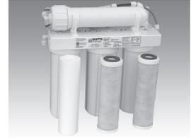
**Step F** – Insert a new sediment filter (cloth like appearance) into the 1st filter housing which is the one on the water inlet side (green tubing from the Adapt-A-Valve™) of the RO system, and re-install housing.
