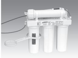
**Step D** – For more leverage you may leave the RO module attached to wall of cabinet. If you are unable to access the module while it is mounted, remove it prior to changing filters. Starting with the closest housing (Stage 1), remove it by turning it clockwise (left), empty water, then discard filter. Continue on to the 2nd housing (Stage 2) and 3rd housing (Stage 3).
