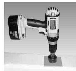
**Step C** – Using a 1/2" hole saw, proceed to drill the large hole. Keep drill speed on the slowest speed and use lubricating oil or liquid soap to keep the hole saw cool during cutting.
