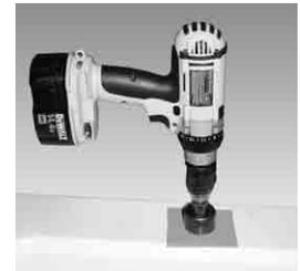
**Step C** – Using a 1¼" hole saw, proceed to drill the large hole. Keep drill speed on the slowest speed and use lubricating oil or liquid soap to keep the hole saw cool during cutting.
