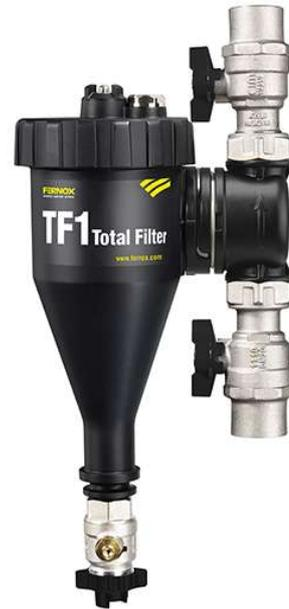
This award-winning TF1 Total Filter combines hydrocyclonic action with powerful Neodymium magnetic assemblies, to remove magnetic and non-magnetic contaminants from system water and contain them safely within the filter. It fits onto vertical and horizontal pipework, can be cleaned in minutes, does not restrict flow in any way.
