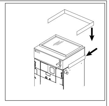
**STEP 4 -** Attach flange to air handler and coil.
