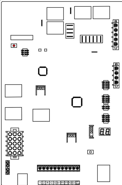
4. If voltage is present in Steps 1 through 3 and the induced draft blower is operating, check for 120 volts to the ignitor during the preheat cycle. Measure voltage between Pin 1 and Pin 5 (on the 5-pin connector) located on ignition control. No voltage, check low stage and high stage pressure switches or replace the ignition control board.
