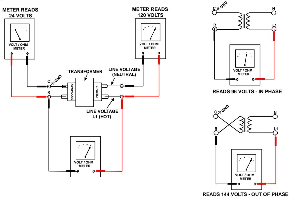
If meter reads approximately 96 volts - the primary to secondary are in phase - if reads approximately 144 volts out of phase - reverse low voltage wires.
