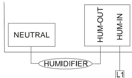
**Wiring Using HUM IN - HUM OUT Terminals**
