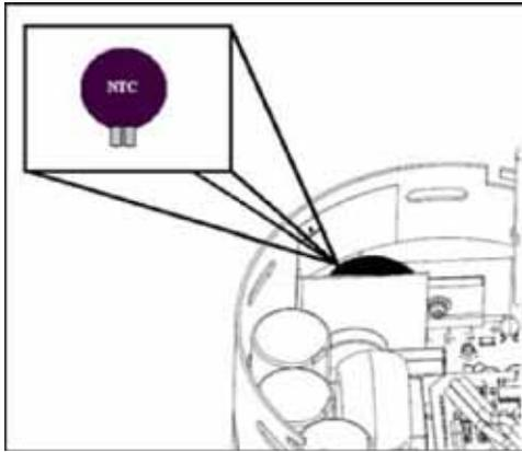
6. Inspect the large capacitors inside the control/end bell (see figure below). Replace the control/end bell if any of the capacitors are bulging or swollen.
