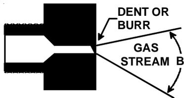
A dent or burr will cause a severe deflection of the gas stream.
