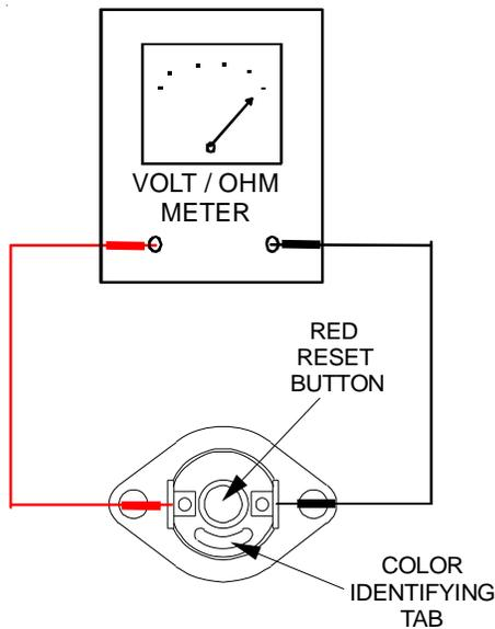
**Testing Auxiliary Limit Control
