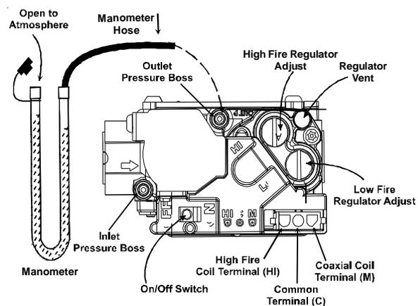
**Measuring Manifold Gas Pressure
