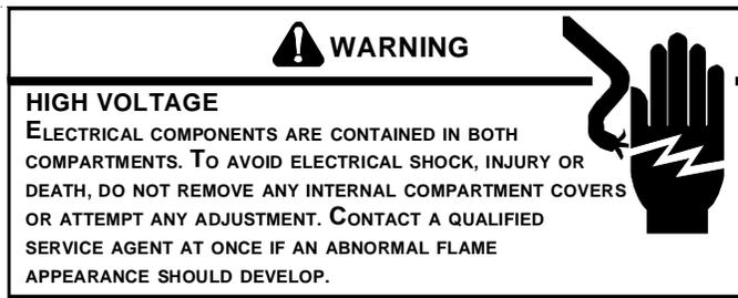
Periodically during the heating season make a visual check of the burner flames. Turn the furnace on at the thermostat. Wait a few minutes since any dislodged dust will alter the normal flame appearance. Flames should be stable, quiet, soft and blue with slightly orange tips. They should not be yellow. They should extend directly outward from the burner ports without curling downward, floating or lifting off the ports.
