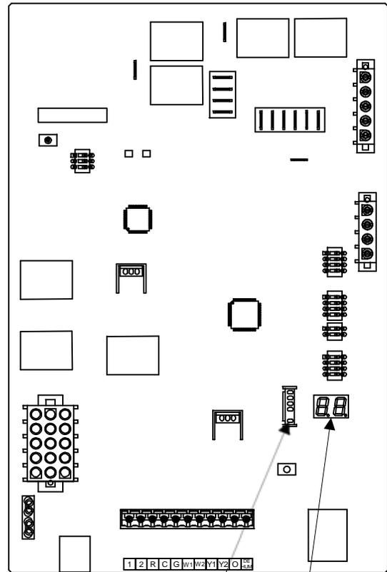
1. **Internal Control Failure with Integrated Ignition Control.** Check for voltage to the furnace and low voltage at the control board. Check for blown fuse on the control board. If the control determines it has an internal fault, it enters a locked-out state. Any of the situations mentioned will cause the dual, 7-segment LED's to be **off**. The control board should only be replaced only after all other checks from the *Troubleshooting Chart - ComfortNet™* have been verified.
