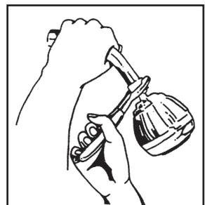
**5** Wrap the shower arm threads with plumber tape before installing into plumbing fitting. Hand tighten hose end to shower arm (or water supply) by turning clockwise. Then fully tighten with an adjustable wrench or pliers. Use a soft cloth between the jaws of the tool and hose connector to protect the finish.
