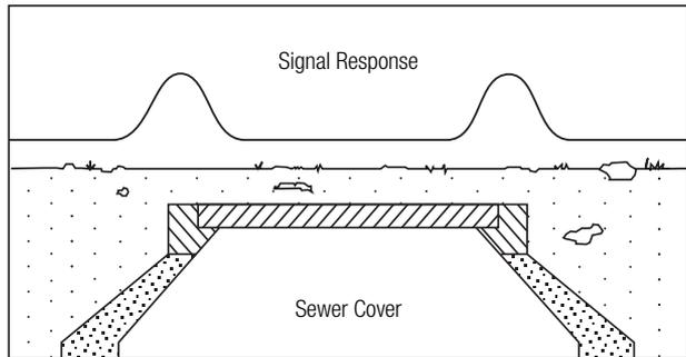
The joints, elbows and ends of iron pipes will create the strongest signals (Fig. 8). Hold the locator in a vertical position while searching to produce the best results.
