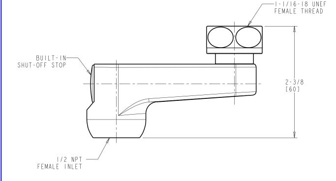
DIMENSIONS ARE IN INCHES AND [MILLIMETERS].
