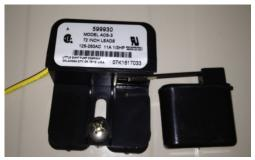
First you need to find a Normally open float switch. The switch we use in this example is a Little Giant model#ACS-3. (Any normally open switch will work) The switch comes normally closed from factory, but needs to be changed to normally open by moving the wire from NC to NO.
