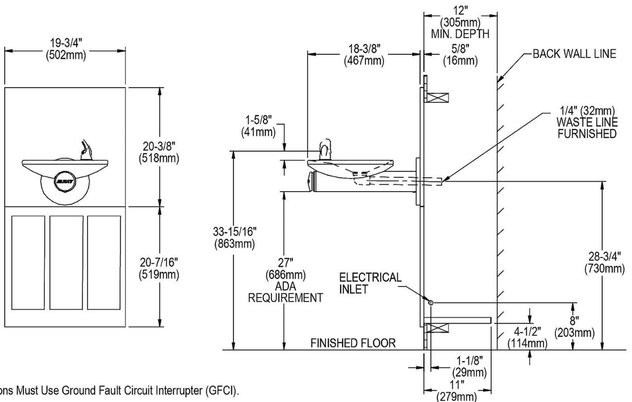
Note : New Installations Must Use Ground Fault Circuit Interrupter (GFCI).
