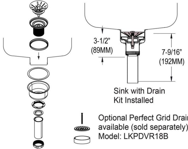
Sink with Drain Kit Installed
