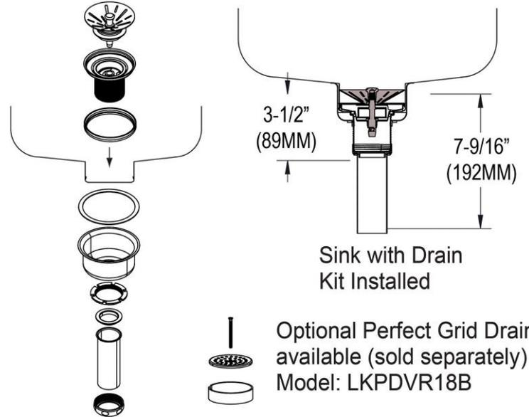
Sink with Drain Kit Installed
