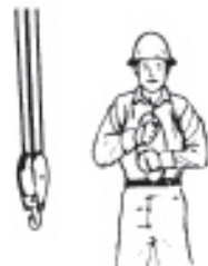
Travel (Both Tracks). Use both fists in front of body, making a circular motion about each other, indicating direction of travel; forward or backward. (For crawler cranes only.)
