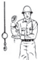
Use Whipline (Auxiliary Hoist). Tap elbow with one hand, then use regular signals.
