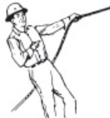
Retract Boom (Telescoping Boom). One Hand Signal. One fist in front of chest, thumb pointing outward and heel of fist tapping chest.
