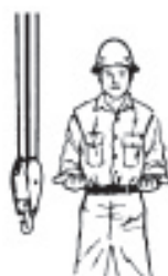
Extend Boom (Telescoping Booms). Both fists in front of body with thumbs pointing outward.
