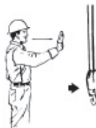
Travel. Arm extended forward, hand open and slightly raised, make pushing motion in direction of travel.
