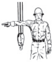
Swing. Arm extended, point with finger in direction of swing of boom.
