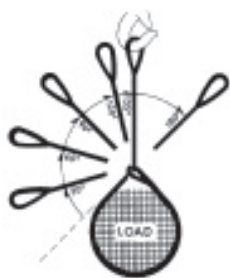
Figure 3. Choker hitch rated capacity adjustment. For wire rope slings in choker hitch when angle is less than 135°.
