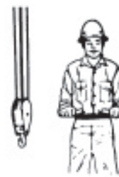
Retract Boom (Telescoping Booms). Both fists in front of body with thumbs pointing toward each other.
