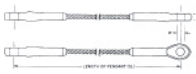
SINGLE ROPE LEGS AND CLOSED SWAGED SOCKETS BOOM PENDENTS WITH SWAGED FITTINGS
