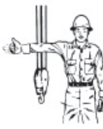
Raise the Boom and Lower the Load. With arm extended, thumb pointing up, flex fingers in and out as long as load movement is desired.
