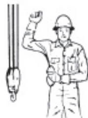
Travel. (One Track). Lock the track on side indicated by raised fist. Travel opposite track in direction indicated by circular motion of other fist, rotated vertically in front of body. (For crawler cranes only).
