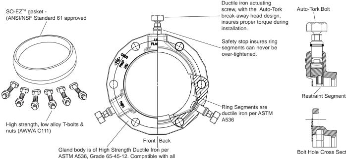
mechanical joints conforming to ANSI / AWWA C111 / A21.11.
