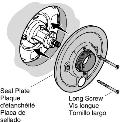
21 Place the escutcheon over the retainer with the notch located at the bottom.
