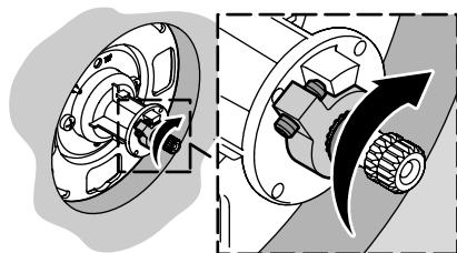
Turn the valve clockwise to the full open position.
