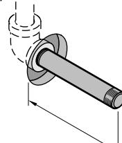
The nipple should extend 4-1/8" (105 mm) past the finished wall.
