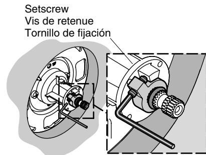
For minor temperature changes, adjust the setscrew and recheck the temperature.
