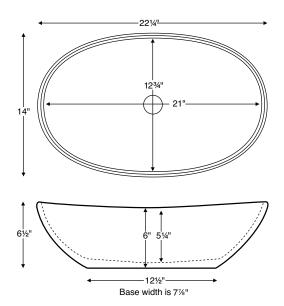
NOTE: Sink rests on top of counter. Cut-out for the drain installation is required. Measurements are ±1/2" and are subject to change without notice. Data herein supersedes all previous prior to publication date indicated below
