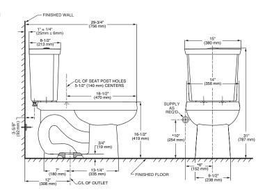
THIS COMBINATION IS DESIGNED TO ROUGH-IN AT A MINIMUM DIMENSION OF 305MM (12") FROM FINISHED WALL TO C/L OF OUTLET. \* DIMENSION SHOWN FOR LOCATION OF SUPPLY IS SUGGESTED. SUPPLY NOT INCLUDED WITH FIXTURE AND MUST BE ORDERED SEPARATELY.
