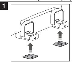
Install rubber base to seat post hinges.
