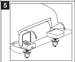
Close the hinge covers. The seat will not work if the hinge covers are not closed tightly.
