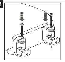
Slip the bolts through the washers, then through the hinge holes.
