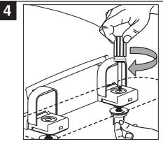
Thread the nuts onto the bolts. Tighten the bolts using a screwdriver. DO NOT OVERTIGHTEN.
