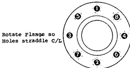
On flanged valves and fittings the flange bolts should be tightened by pulling down the nuts diametrically opposite each other and in the order as numbered (see illustration). All bolts should be pulled down gradually to a uniform tightness. Uniform stress across the entire cross section of the flange eliminates a leaky gasket.
