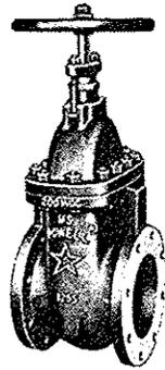
The bonnet and body neck flanges are bolted together. This type of stem design is generally used in gate valves. The stem rotates and threads into a disc holder that is threaded into the disc. The stem does not rise but merely turns with the handwheel. Non-rising stem valves are ideally suited where headroom is limited.
