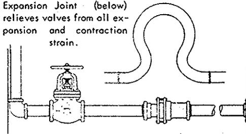
Frequently, on large size high-pressure high-temperature steam lines or lines carrying hazardous media, a "U" Bend welded in the line serves the same purpose.
