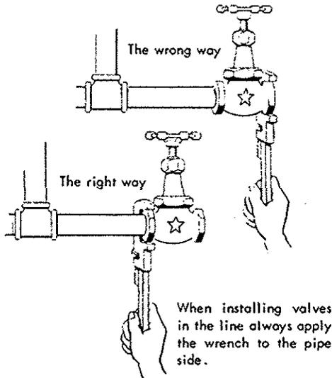
When installing threaded end valves always use the proper size wrenches with flat jaws (not pipe wrenches). By so doing there is less likelihood of the valve being distorted or damaged. Also the wrench should be used on the pipe side of the valve to minimize the chances of distorting the valve body. This is important where the valve is made of a malleable material, such as bronze. As a further precaution against distortion, see that the valve is closed tightly before it is installed.
