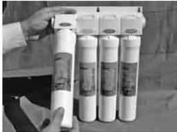
**Step C** – Make sure to remove the cap off of the new replacement filter. Insert the new filter cartridge into the head and rotate it clockwise ¼ turn until it stops. Return cartridge to the vertical position.
