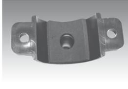
**Step C** – The drain saddle must be installed at least 1 1/2" above the nut of the P-Trap elbow or cross bar from the garbage disposal to insure proper drainage. Using the 1/4" drill bit, drill into the drain pipe at best available location as specified above, for drain saddle installation. Take extreme caution to only drill through one side of the drain pipe.
