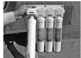
**Step D** – Repeat this procedure for the 2nd, 3rd and 4th filter cartridges. When finished, flush your tank completely once to remove any natural carbon fines from the RO system. Check over the next 24 hours to ensure no leaks are present.
