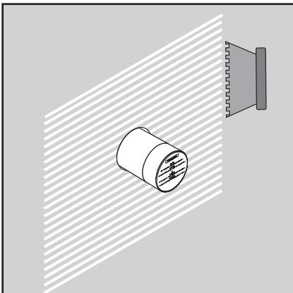
Apply adhesive (not included) to the wall around the valve.
