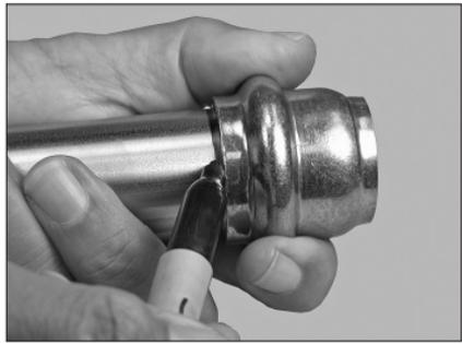
2. While the pipe is inserted completely into the gauge, mark the pipe along the edge of the gauge with a marker or paint stick, as shown above.
