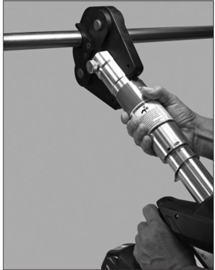
Press Ring/Vic-Press Adapter Jaw Assembly for 1½-inch/48.3-mm and 2-inch/60.3-mm Sizes
