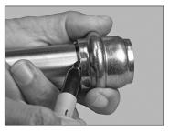
**2.** While the pipe is inserted completely into the gauge, mark the pipe along the edge of the gauge with a marker or paint stick, as shown above.
