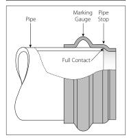
**1.** When using the Vic-Press Schedule 10S Marking Gauge, insert the pipe end into the correct size gauge. Make sure the pipe end contacts the pipe stop (refer to the sketch above).
