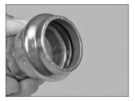
1. Check the openings of Vic-Press Schedule 10S System Products to make sure seals are seated properly inside the seal pocket. Verify that the seals are a material grade that is compatible with the intended service.
