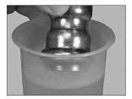
IF PRODUCT IS NOT SHIPPED FROM THE FACTORY IN A BAG, THE SEALS ARE NOT PRE-LUBRICATED AND MUST BE LUBRICATED IN THE FOLLOWING MANNER. Lubrication is essential to prevent seals from being pinched during installation. Fittings should be dipped into a soapy water solution. Make sure the seals are wetted thoroughly, and complete all pressing steps while the seals are still wet.
