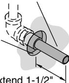
The tube should extend 1-1/2" (38 mm) - 2-7/8" (73 mm) past the finished wall.
