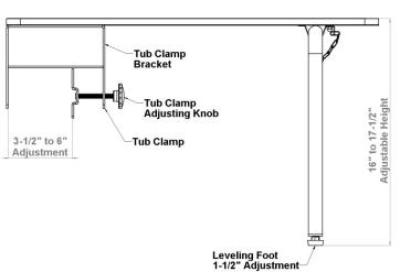
Holding the Bench in its horizontal position in the tub, adjust the Tub Clamps so they will fit over the front of the tub ledge.
