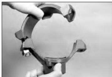
**1. ASSEMBLE HOUSINGS:** Insert a bolt into the two housings. Thread a nut loosely onto the bolt (nut should be flush with end of bolt).
