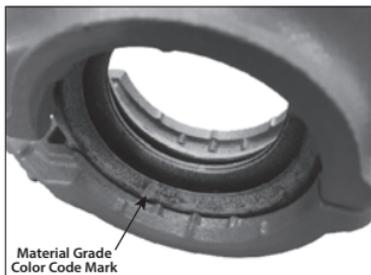
**3. CHECK GASKET:** Check the gasket to verify that it is suitable for the intended service. The color code identifies the material grade. Refer to page 32 for the "Gasket Color Code Reference" table and the "NOTICE" on page 36 for important gasket information. For complete compatibility information, reference Victaulic publications 05.01 and GSG-100, which can be downloaded at victaulic.com.
