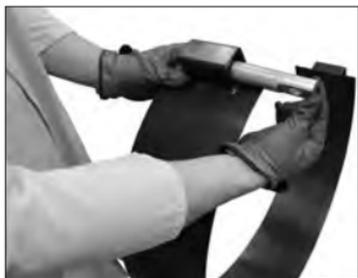
**1. INSERT CROSSBAR:** Insert a crossbar into the retaining bracket on both sides of the strap. The flat side of the crossbar shall face away from the open end of the strap, as shown in the profile view in step 3 below.
