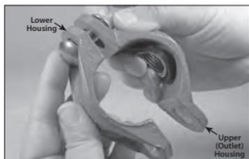
**2. ASSEMBLE HOUSINGS:** Remove the flange nut and bolt from one side of the Style 912 assembly. Thread the remaining flange nut loosely onto the bolt (flange nut should be flush with end of bolt) to allow for the "swing-over" feature.
