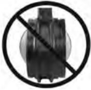
**DO NOT INSTALL BUTTERFLY VALVES INTO THE SYSTEM WITH THE DISC IN THE FULLY-OPEN POSITION. Exposed disc may be damaged and prevent proper function of the valve.**
