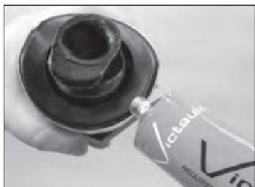
**3b. LUBRICATE GASKET:** DO NOT REMOVE THE GASKET FROM THE STYLE 923 OR 924. Apply a thin coat of a compatible lubricant ONLY to the exposed sealing surface of the gasket. Refer to the “Lubricant Compatibility for Gaskets” table on page 34.
