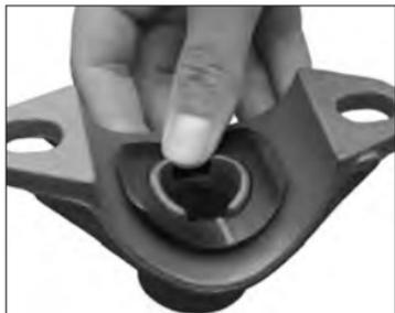
**1b. INSTALL GASKET:** Inspect the gasket and the gasket pocket to verify that no debris is present. Install the gasket into the gasket pocket, as shown. Press the gasket along the full circumference to ensure that it seats fully in the gasket pocket. **DO NOT LUBRICATE THE GASKET.**
