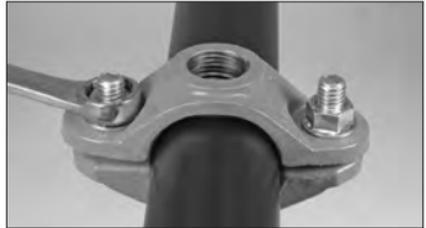
**5. TIGHTEN FLANGE NUTS:** Verify that the locating collar is still positioned properly in the outlet hole. Tighten the flange nuts evenly by alternating sides, maintaining nearly uniform bolt pad gaps, to a maximum torque value of 20 ft-lbs/27 N•m to ensure proper gasket compression. Verify that the oval neck of each bolt seats properly in the bolt holes. Refer to the “Helpful Information” table below.
