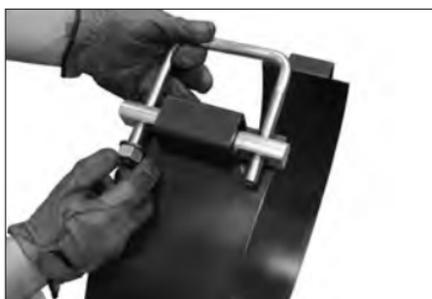
**3. LOOSELY THREAD NUTS:** Place one washer over each end of the U-bolts, then loosely thread a nut over each washer. The nuts should only be tight enough to hold the assembly in place.
