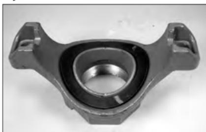
**2. CHECK GASKET:** Check the gasket to verify that it is suitable for the intended service. The color code identifies the material grade. Refer to page 32 for the “Gasket Color Code Reference” table. For complete compatibility information, reference Victaulic publications 05.01 and GSG-100, which can be downloaded at [victaulic.com](http://victaulic.com). Inspect the sealing surface of the gasket to verify that no debris is present.
