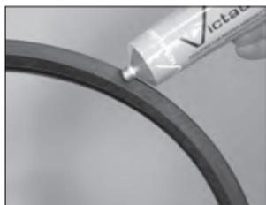
**6. LUBRICATE GASKET:** Apply a thin coat of a compatible lubricant to the gasket sealing lips and exterior. Refer to the “Lubricant Compatibility for Gaskets” table on page 34.
