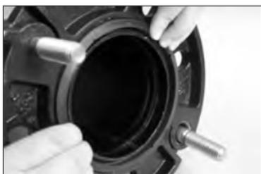
**6c.** Verify that the Flange Gasket is still seated properly within the gasket pocket of the Style 741, 841, 743, or 744 and that the lettering on the Flange Gasket is not visible when viewing the face of the Style 741, 841, 743, or 744.
