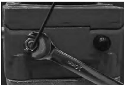
**4a.** Using a hex key wrench, tighten the internal set screw (clockwise) until it contacts the internal quadrant gear.
