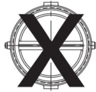
Incorrect Orientation for Horizontal Installation
