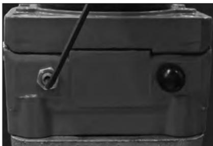
**2a.** Loosen the hex lock nut (counterclockwise) located on the left side of the gear operator.
