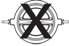
Incorrect Orientation for Horizontal Installation
