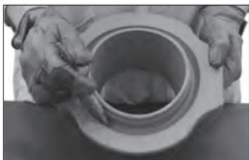
**4. LUBRICATE GROOVE:** Apply a thin coat of a compatible lubricant **ONLY** to the o-ring groove on the underside of the spigot housing. Refer to the “Lubricant Compatibility for Gaskets” table on page 34. When using the Style 926 with HDPE pipe, always consult the pipe manufacturer for lubricant compatibility requirements.
