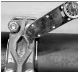
**10. TIGHTEN NUTS:** Using an impact tool or a standard socket wrench with a deep-well socket, tighten the nuts evenly by alternating bolt pad locations until the gaps are equal at all bolt pads. Verify that the oval neck of each bolt seats properly in the bolt holes. **To complete the assembly, apply torque to each nut with a torque wrench.** Refer to the “Assembly Torque Requirements” table on the following page and the “Torque Wrench Selection” section in this handbook.
