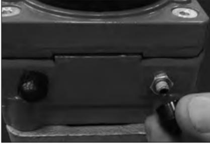
1. Remove the dust cap from the right side of the gear operator.
