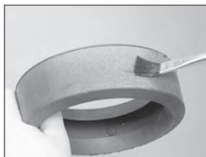
**5. LUBRICATE GASKET:** Apply a thin coat of a compatible lubricant to the gasket sealing lips and exterior. Refer to the “Lubricant Compatibility for Gaskets” table on page 34.
