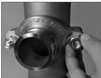
**6. INSTALL REMAINING BOLT/NUT:** Insert the remaining bolt. Thread a nut onto the bolt finger-tight. **NOTE:** Verify that the oval neck of each bolt seats properly in the bolt hole.
