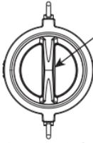
Correct Orientation for Horizontal Installation
