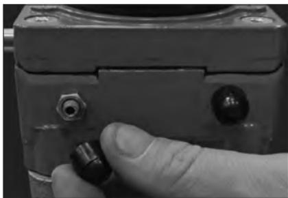
**1.** Remove the dust cap from the left side of the gear operator.
