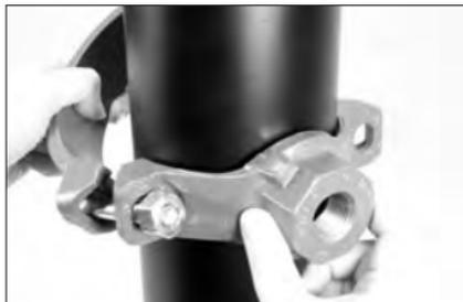
**4. INSTALL HOUSINGS:** Rotate the lower housing so that it is positioned approximately 90° to the upper (outlet) housing, as shown above. The upper (outlet) housing's locating collar shall be placed into the outlet hole. Rotate the lower housing around the pipe.
