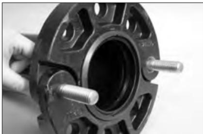
**6b.** Insert a standard full-shank-diameter assembly bolt through the two lap-joint bolt hole locations, as shown above. Refer to the applicable “Helpful Information” table on pages 212 – 215 for the required assembly bolt size and length. **NOTE:** Victaulic does not supply these assembly bolts.
