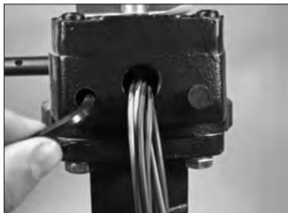
3a. Using a hex key wrench, loosen the internal set screw counterclockwise.
