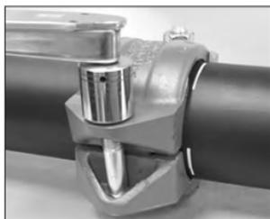
**10. TIGHTEN NUTS:** Using an impact tool or a standard socket wrench with a deep-well socket, tighten the nuts evenly by alternating sides until the gaps are equal at the bolt pads. Verify that the oval neck of each bolt seats properly in the bolt holes. **To complete the assembly, apply torque to each nut with a torque wrench.** Refer to the “Assembly Torque Requirements” table on the following page and the “Torque Wrench Selection” section in this handbook.
