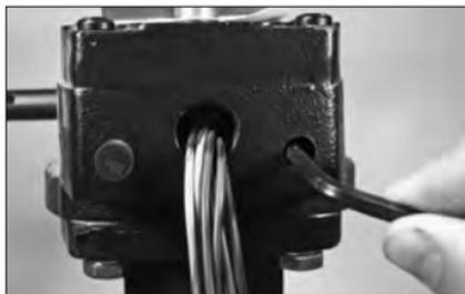
4. With the valve disc in the fully “SHUT” position, tighten the internal set screw (clockwise) with a hex key wrench.
