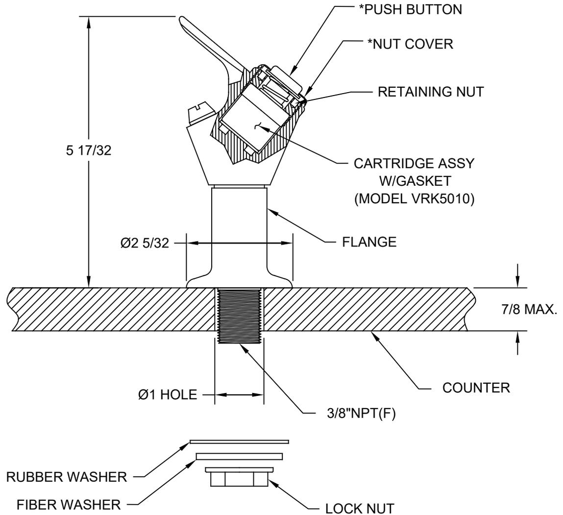
\*CHROME PLATED PUSH BUTTON COVER & NUT ARE STANDARD ON 5010.6427SS. COPPER PLATED OPTION IS AVAILABLE AS MODEL PB8C.
