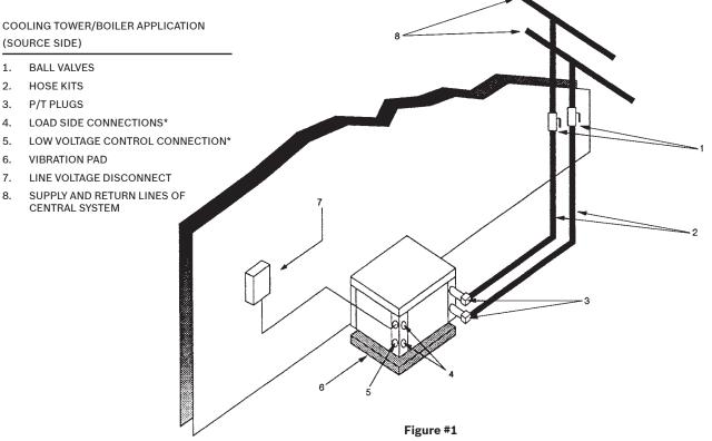
\* NOTE: Water and electrical connection locations vary depending on model. Connect as required per unit labels.
