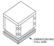
If the unit is installed on a floor over a crawl space, it should not rest on long, unsupported floor joists. Vibrations may be created in the joists with the crawl space acting as an amplifier box resulting in undesirable noise. A drain pan is recommended where water released during start-up or maintenance could cause damage below the unit.
